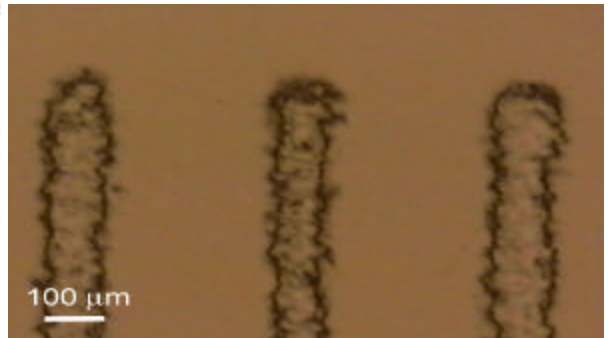
Figure 7: Optical micrograph of photoresist after exposure and development through Kodak TMY200 mask
